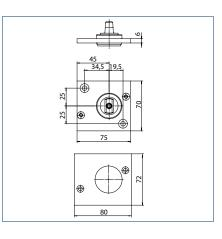
Pivot bearing with flat conical spindle
