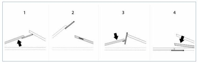
1 = double leaf door opens via the passive leaf | 2 = active leaf is held in the waiting position | 3 = passive leaf closes | 4 = the active leaf is released as soon as the passive leaf is closed
