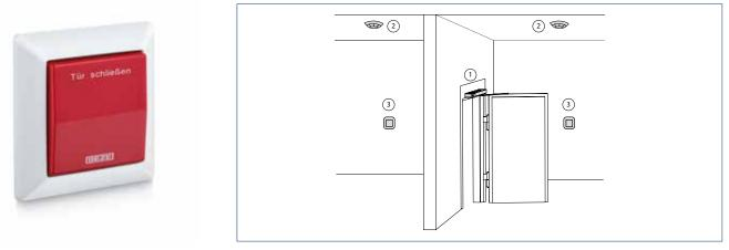
1 = lintel-mounted detector | 2 = ceiling-mounted detectors | 3 = manual trigger switch
