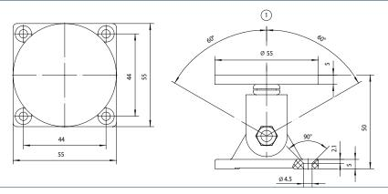
Magnetic counter plate with joint
