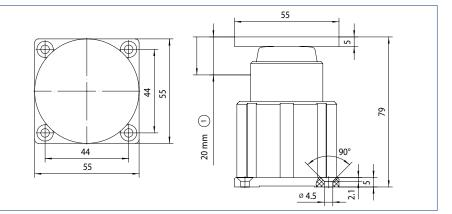
Magnetic counter plate with spring buffer on mounting plate with damping spring for soft-spring-mounted end stop for heavy doors I 1 = 20 mm spring deflection
