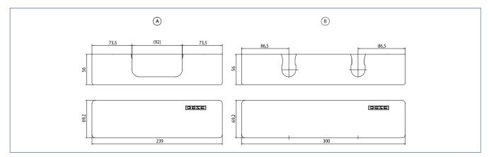
A = cover cap TS 3000/TS 2000 | B = cover cap TS 5000/TS 5000 L/TS 4000
