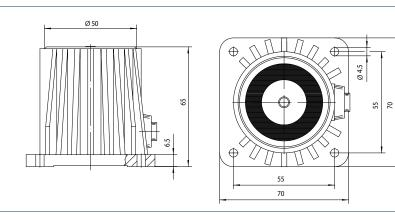
Hold-open magnet wall installation
