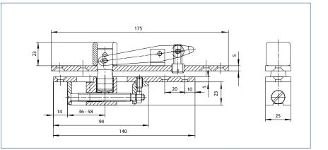
Adjustable pivot hinge model C
