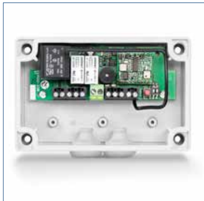
WRM-230B receiving module in IP-54 housing
